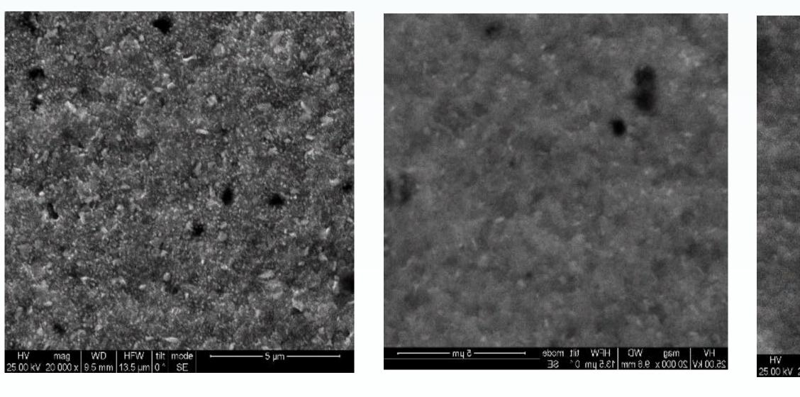
SEM images of CsCH<sub>3</sub>NH<sub>3</sub>Pbl<sub>x</sub>Br<sub>3-x</sub> perovskite and co-sensitized perovskite-QDs PbS/CsCH<sub>3</sub>NH<sub>3</sub>Pbl<sub>x</sub>Br<sub>3-x</sub>, CdS/CsCH<sub>3</sub>NH<sub>3</sub>Pbl<sub>x</sub>Br<sub>3-x</sub> films.
