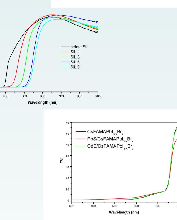
UV- Vis T% spectra of QDs , perovskite and co-sensitized perovskite-QDs films. The perovskite and the co-sensitized perovskite-QDs curves are similar, although PbS/CsFAMAPbl3-xBrx seem to have the best absorbance
